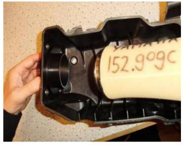
7. Secure airboot to the plastic flange:
